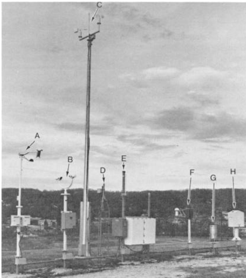
Figure 2-1.—ASOS sensors: A. Visibility sensor; B. present weather sensor; C. wind direction and wind speed sensor; D. freezing rain sensor; E. DCP antenna and data collection package (equipment case); F. temperature and dew-point sensors; G. rain gauge; and H. cloud height sensor.
