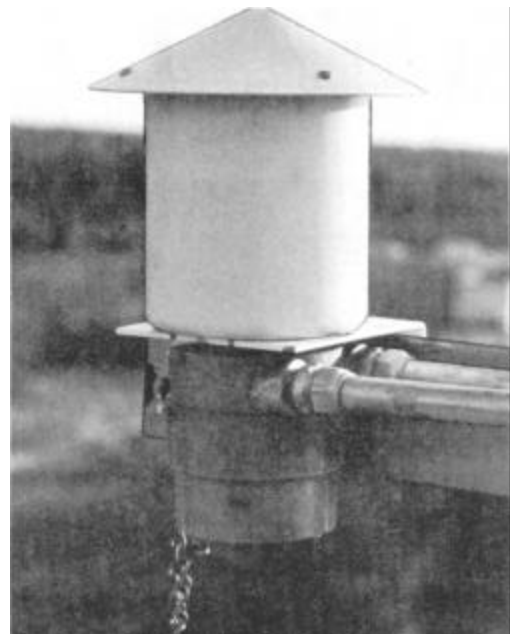
Figure 2-11.—ML-643/GMQ-29 dew-point sensor.
